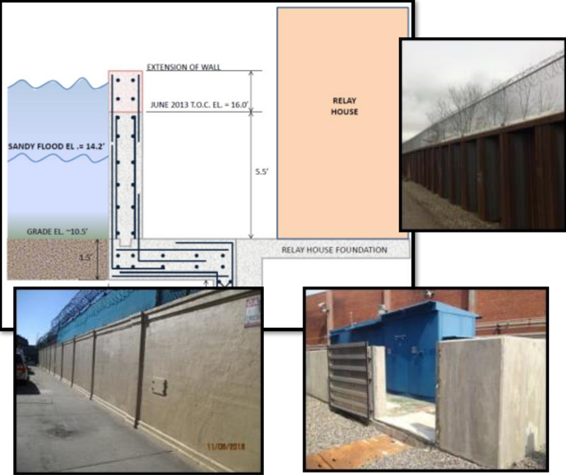
Floodwalls designed to FEMA 100-year flood levels +3 feet protect critical infrastructure
